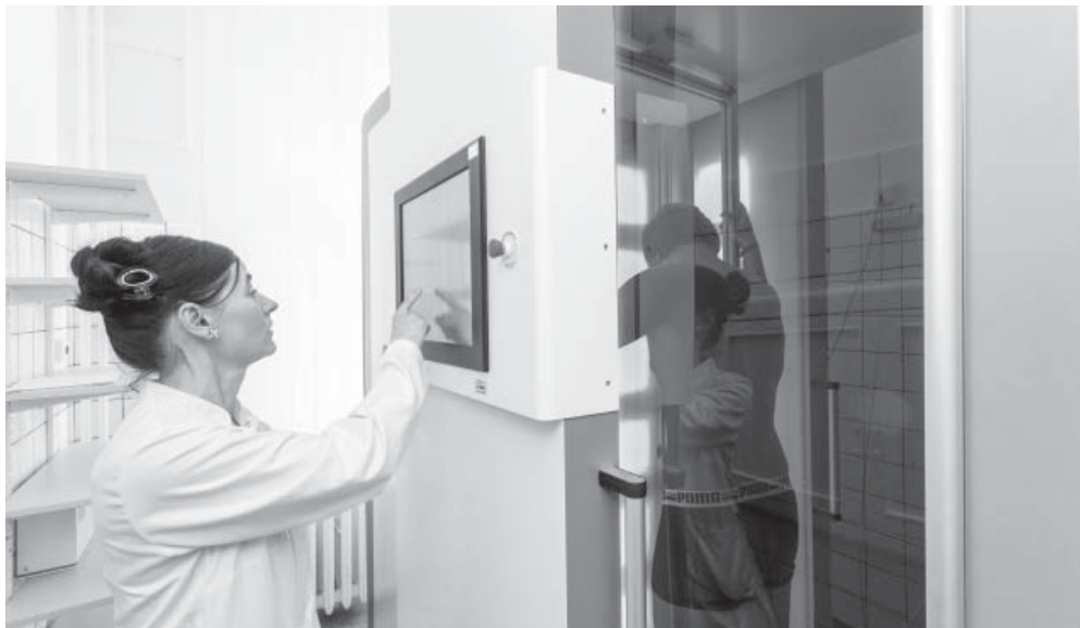
The Dermascanner scans the surface of a patient's skin from different positions and divides it into around one hundred individual images. (© Dirk Mahler/Fraunhofer IFF) | Picture in color and printing quality: www.fraunhofer.de/press
